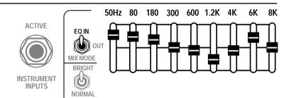
To activate the 9 Band Equalizer via the Footcontroller, you must have the front panel 3 position mini toggle switch in the OUT position or in the MIX MODE position. There are two of these switches, one per channel located to the right and left respectfully. When the E.Q. 3 position switch is in the MIX MODE, the E.Q. will automatically be engaged.
